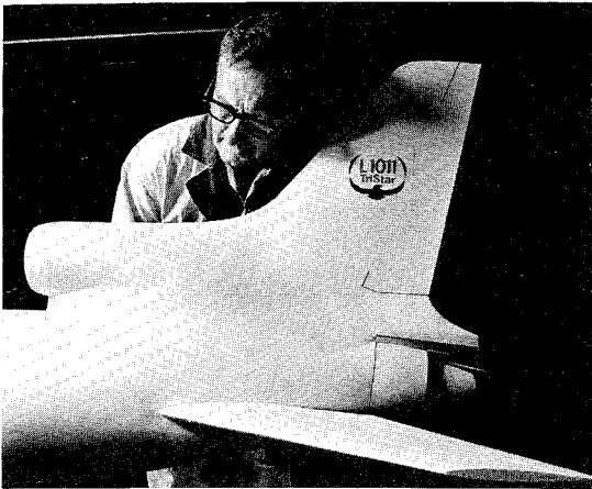
Fig. 10 Model with flowing inlet and jet.
